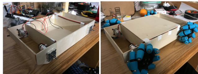
Figure 16: Printed Wheel Parts and Assembly
